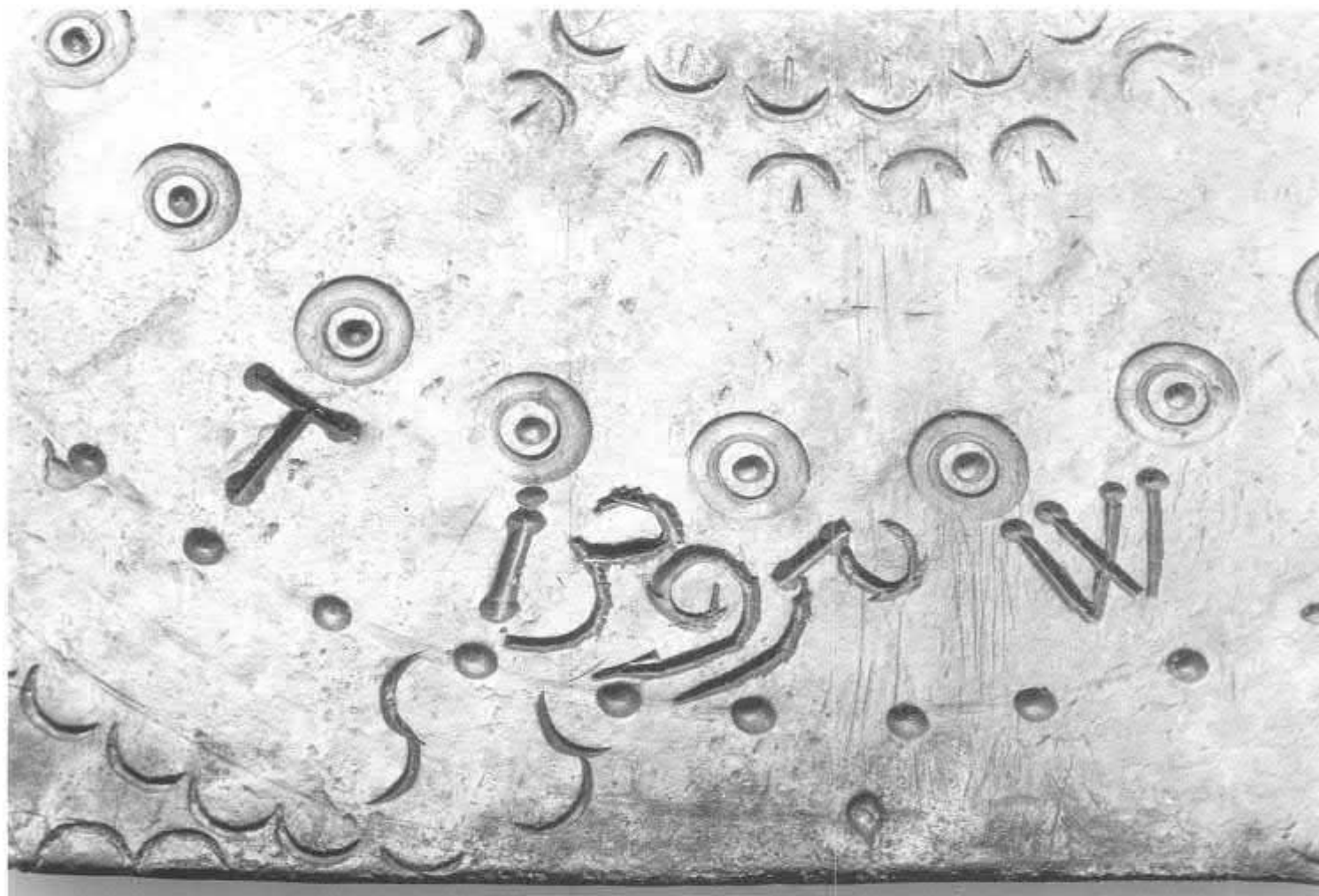
FIGURE 5 Close-up photograph showing the detail of the punched initials 'T.' / 'W.' and the numerals '1395' chiselled into the underside of the dial-plate. The initials may be those of the original maker, diallist, or patron. The date is probably an error that caused the instrument to be reversed and engraved on the other side.
