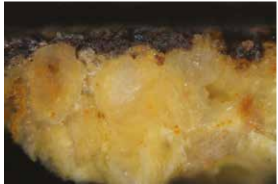
FIGURE 15. Paint sample 05 (voussoir 14), taken from the dark outer band, originally in red. In some places, detail was applied over this in calcium carbonate white (EH)
