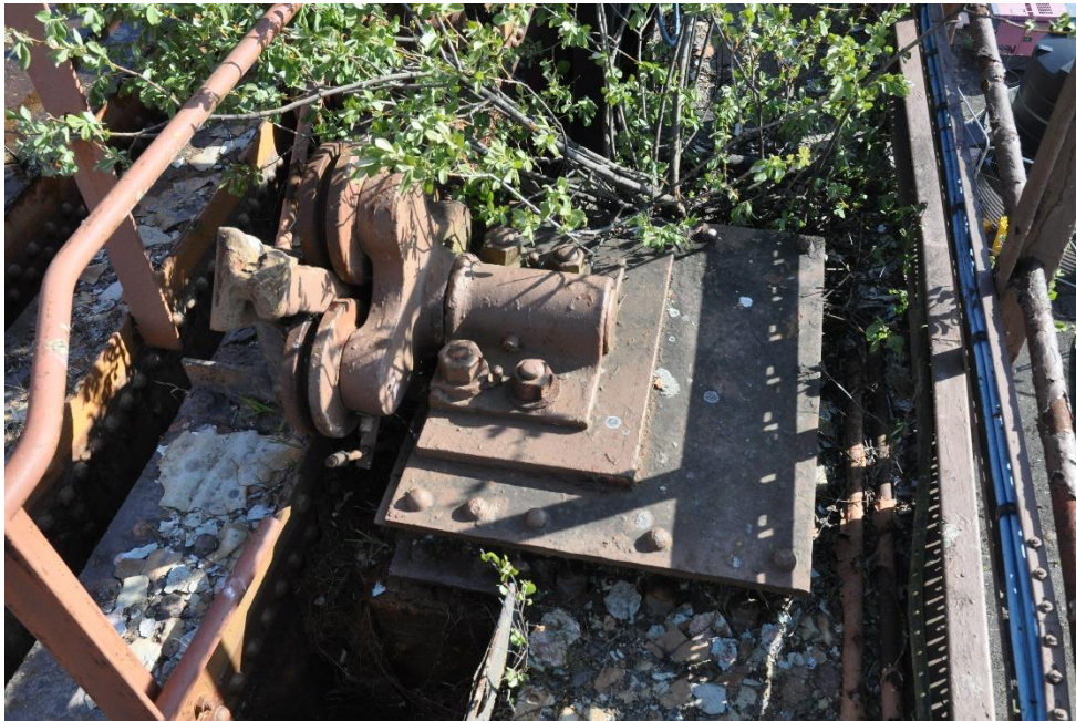
Figure 12: Example of the tank roller carriages.
