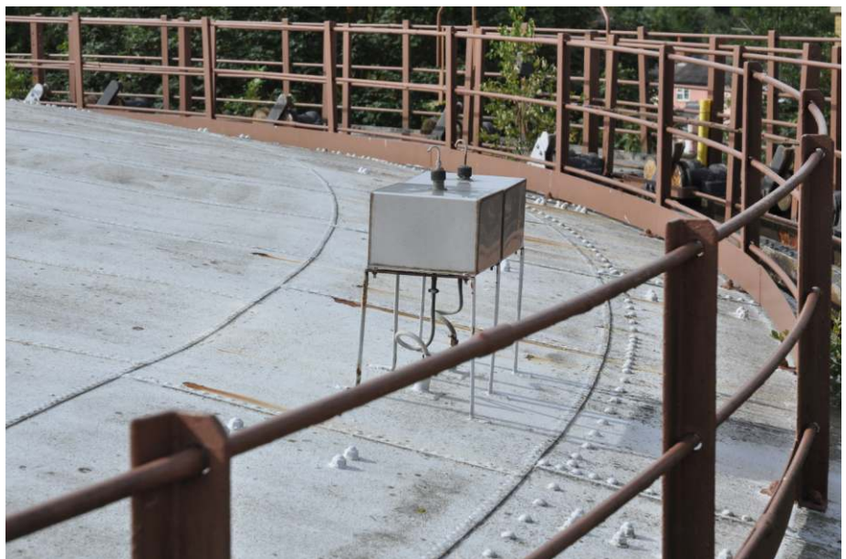
The crown edge with hydrostatic tanks Fig 25
