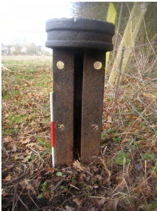
Image 15: Detail of back of rail forming marker, showing hollow, which allowed rail to cool more evenly during manufacture. Scale 0.3m in 10cm divisions.
