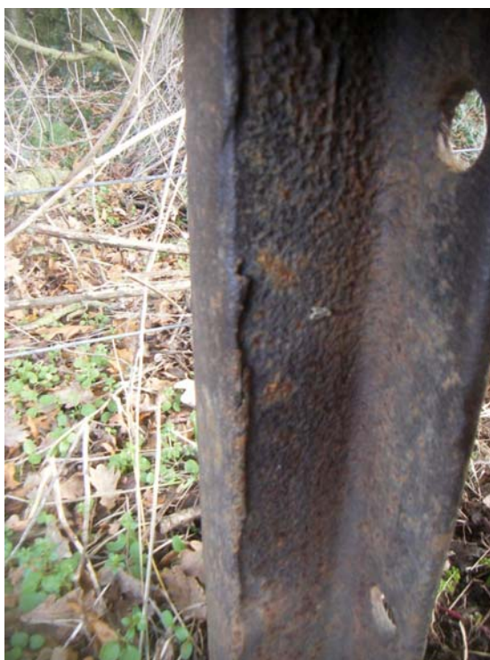
Image 16: Detail of upper part of rail showing deformation; probably due to use.
