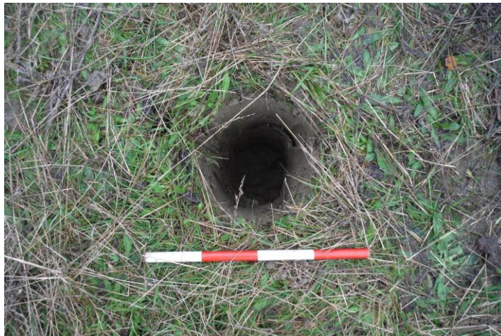
Hand-dug portion of Borehole 3 (40cm scale)
