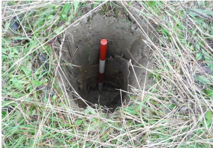
Hand-dug portion of Borehole 1 (40cm scale)
