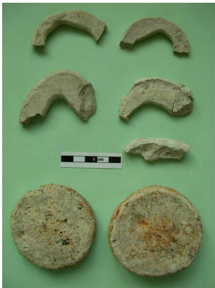
Image 13: Selection of pieces of kiln furniture – ‘ring wads’ and ‘buns’ recovered from the clay tobacco pipe kiln. All the pieces are made from pipe clay. Scale 5cm in 1cm divisions.
