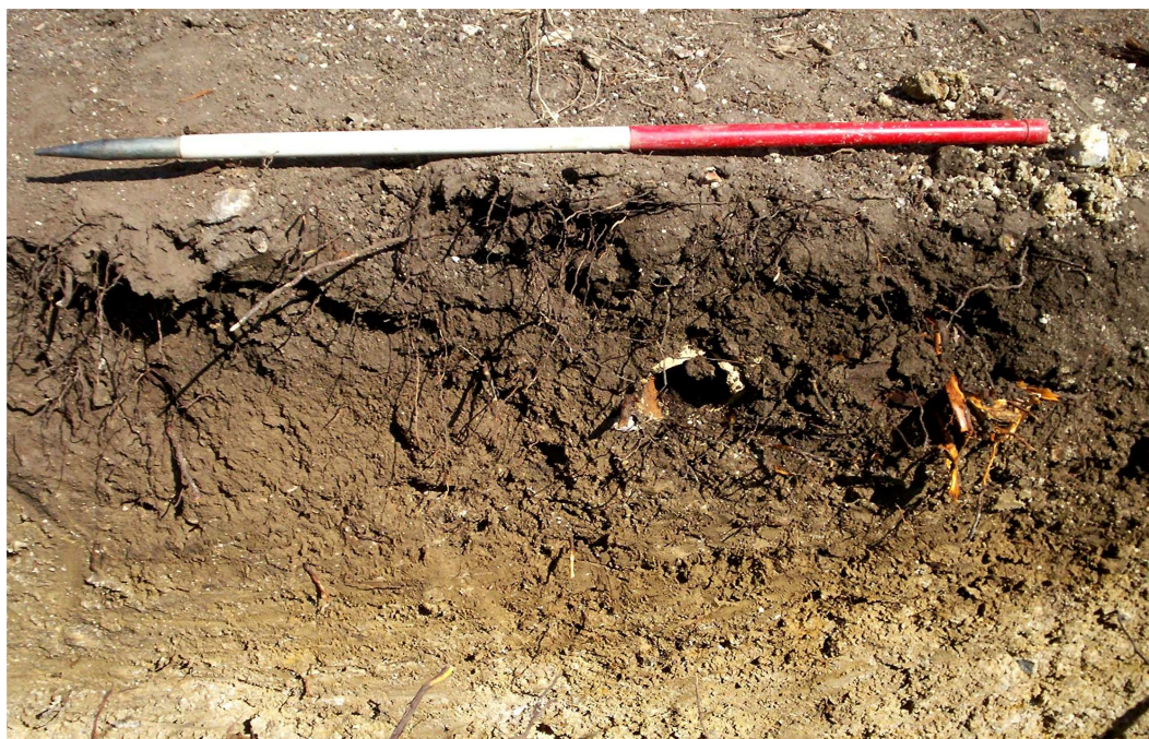
Image 3: Typical soil profiles, with ceramic drain associated with rainwater drainage system. Scale 1m in 50cm divisions.
