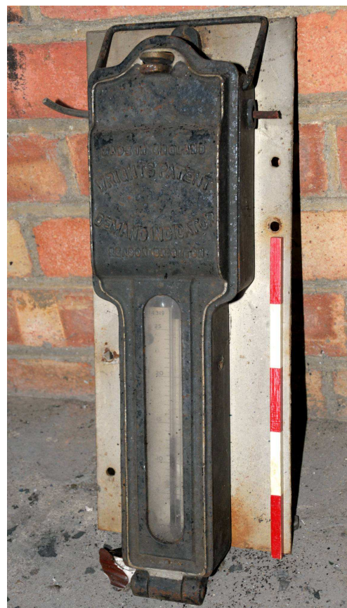
Image 28: Wright's Patent Demand Indicator Shown with cover open at left and closed at right (scale 25cm).
