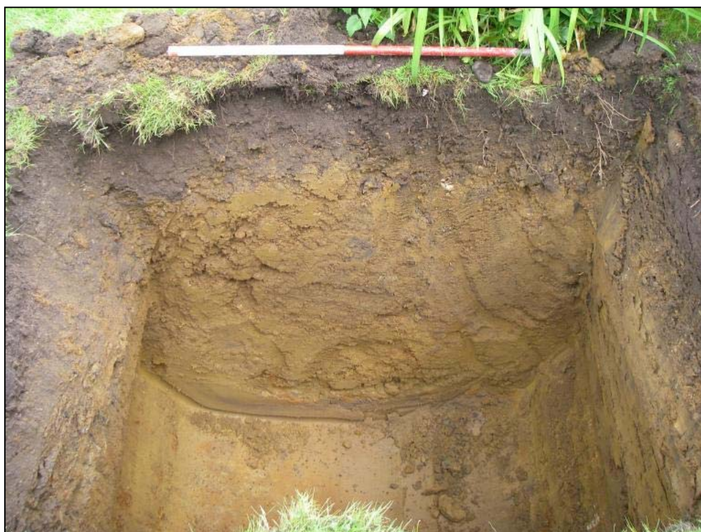
Figure 4: Soil profile in soakaway pit
