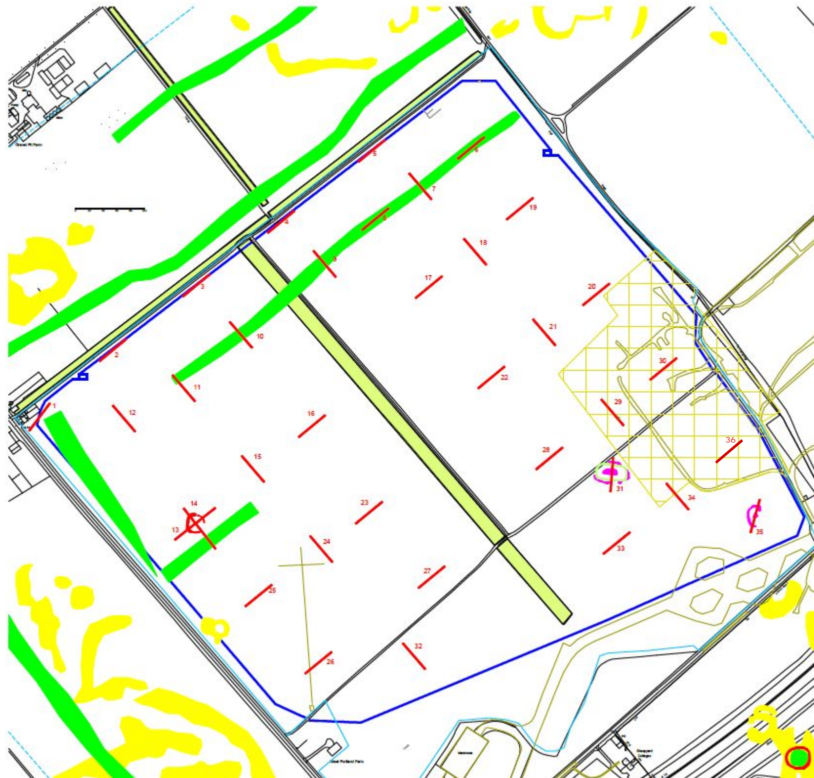
Figure 3: Trench locations on cropmark plot
