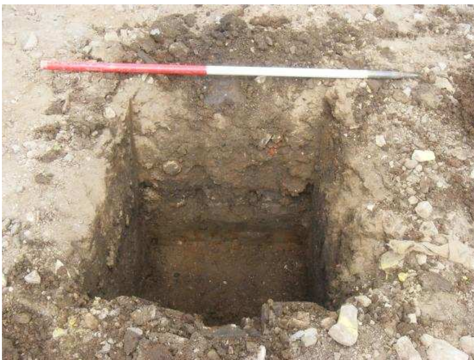
Typical made ground encountered in foundation pits around the former swimming pool
