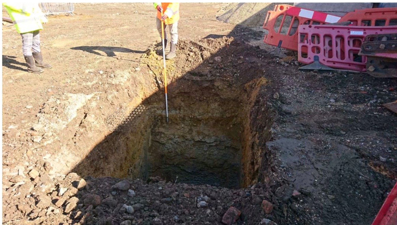
Photograph 7: Test-pit 8, south wing, showing natural sand and gravel deposits at c.28.2m AOD
