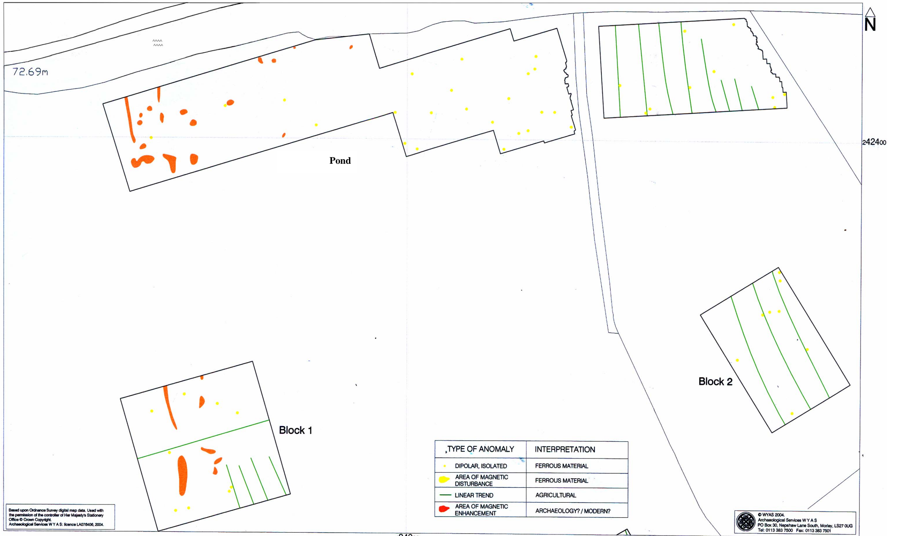
Figure 9: Interpretation of gradiometer data; Pond and Blocks 1 and 2
