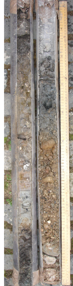
BH7: cores from 1.2–3m (left to right). An organic silt horizon is present at the base of core 1
