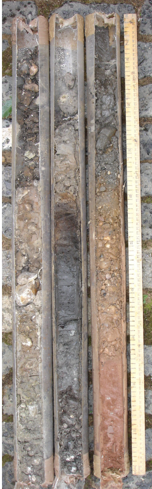
BH1: cores from 1.2–4.0m depth (left to right). Peats are present in the centre of the second core.
