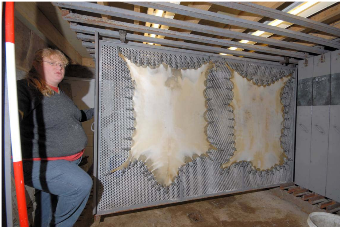
Plate 31: The process: drying cabinet, area F
