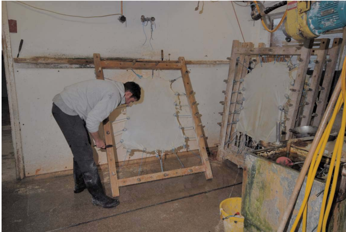
Plate 30: The process: stretching frames
