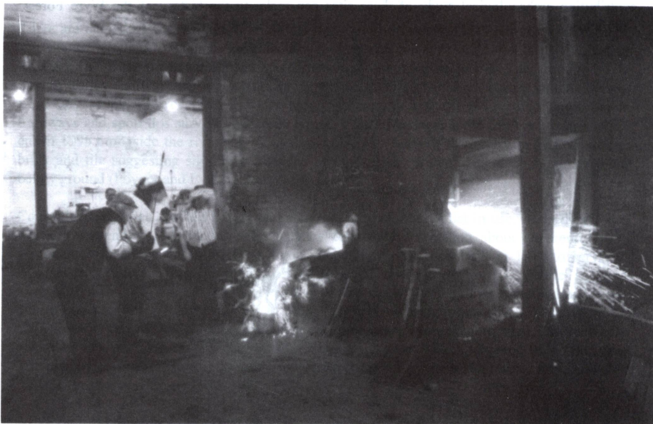
Plate 2: Casters collecting the molten metal from the cupola
