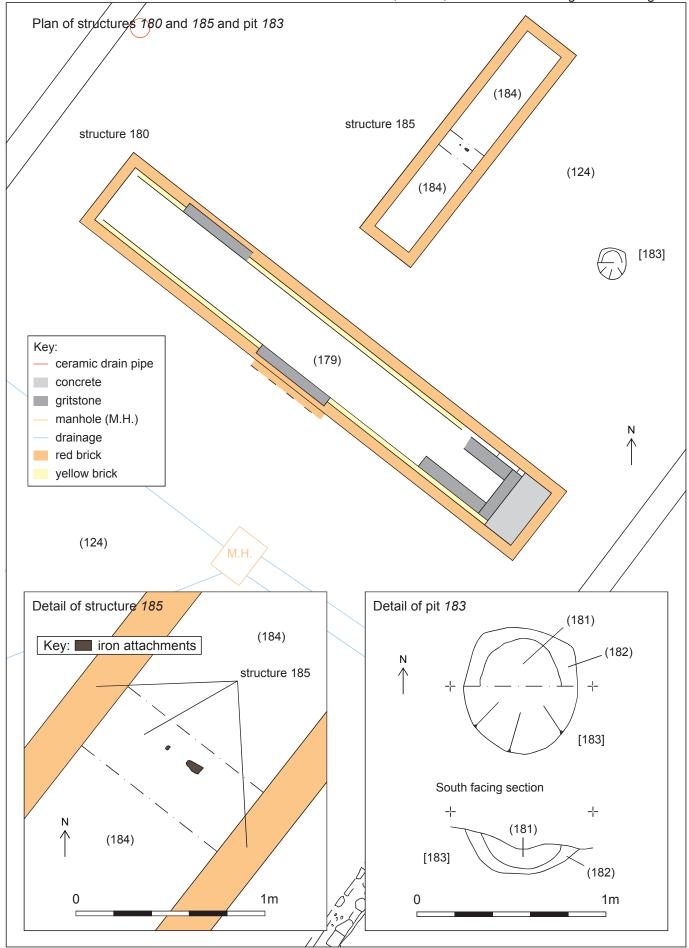
Figure 6: Structures 180 and 185 and pit 183
