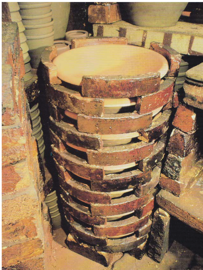
Plate 18: Pan rings in use for the beginning of a bung of pancheons in the kiln at Soil Hill, 1964 (McGarva 2000, 103)
