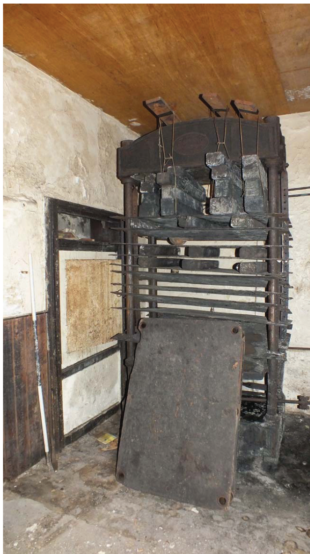
Plate 43 (left): Extant steam press in Room G7, with safe built into the wall to the north Plate 44 (right): Scar and fittings of former steam press against the west elevation of Room G7
