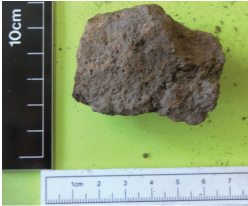
Plate 1 Small piece of viscous smelting slag from Context 1003.
