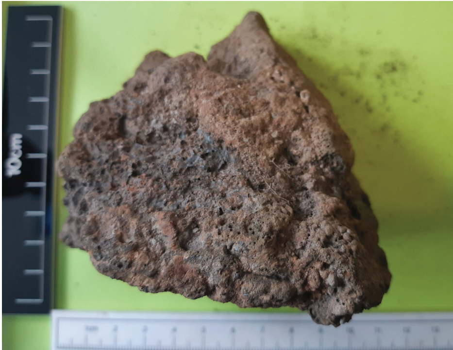
Plate 3 Larger piece of viscous smelting slag, showing rim of furnace lining, (top right to bottom right) edge.
