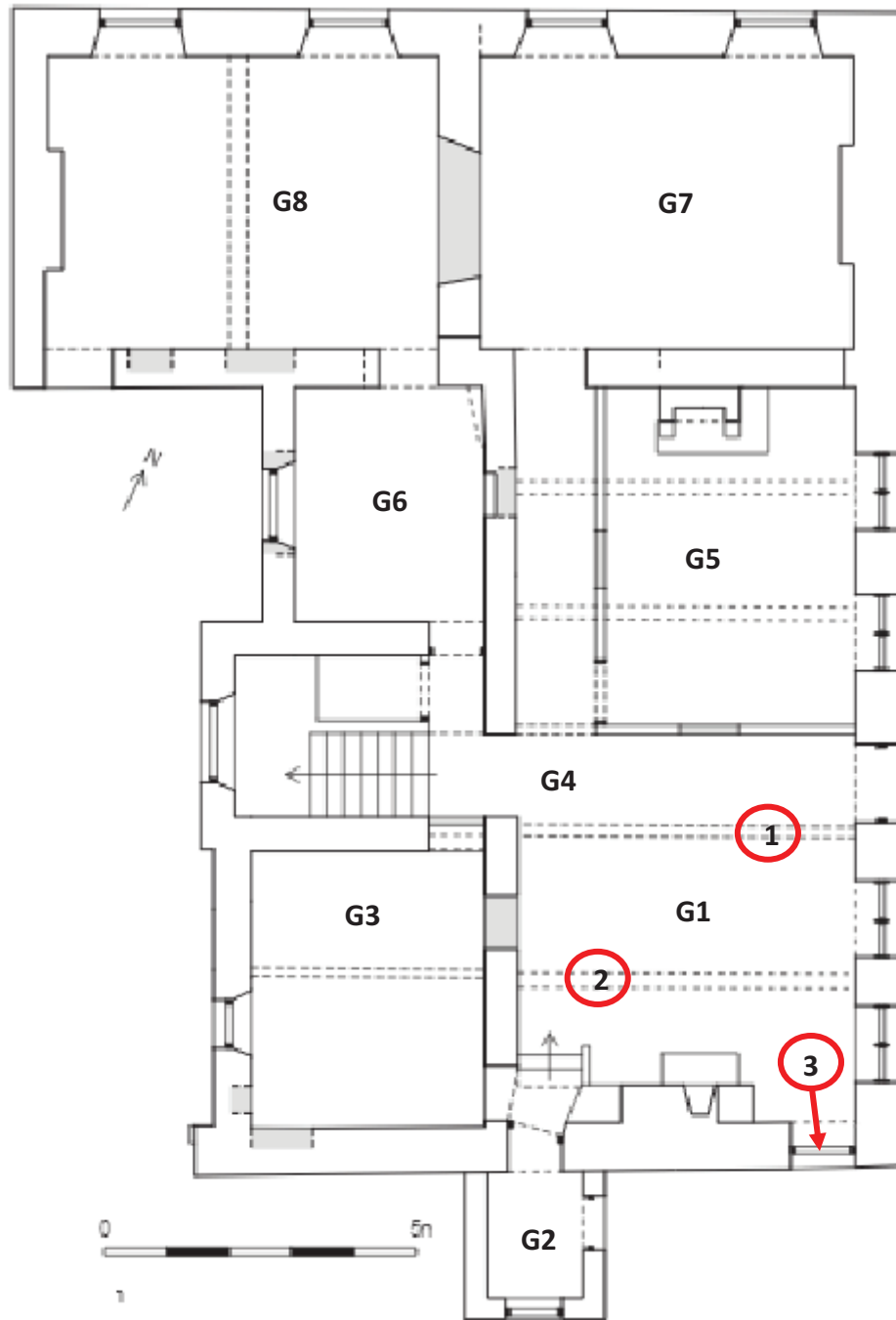
Figure 3a: Plan of ground floor rooms to help locate sampled timbers (see Table 1) (after Greenlane Archaeology Ltd)
