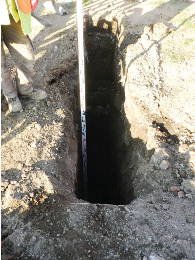
Photo 1 Coal-ash fills in TP1 looking north
