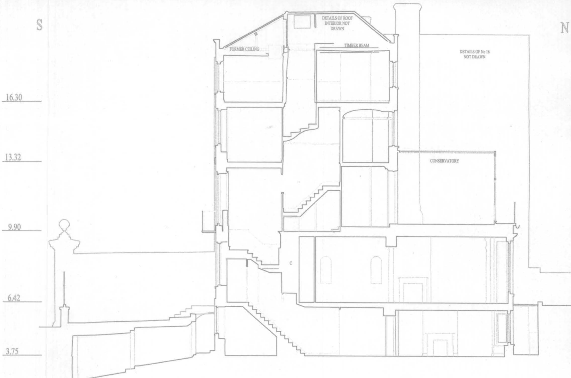
Fig 12 Sectional elevation from south to north through western third of building, looking west (1:100)
