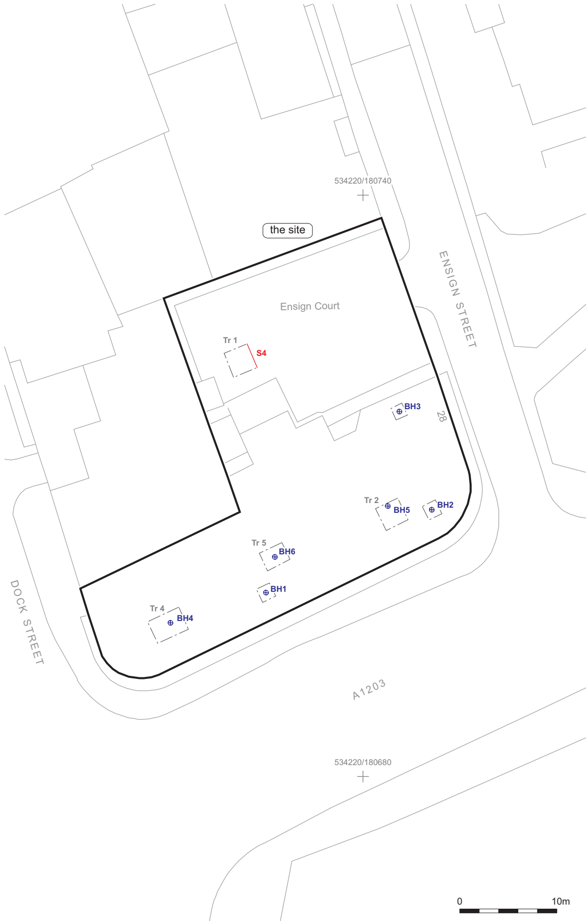
Fig 2 Trench, borehole and section locations
