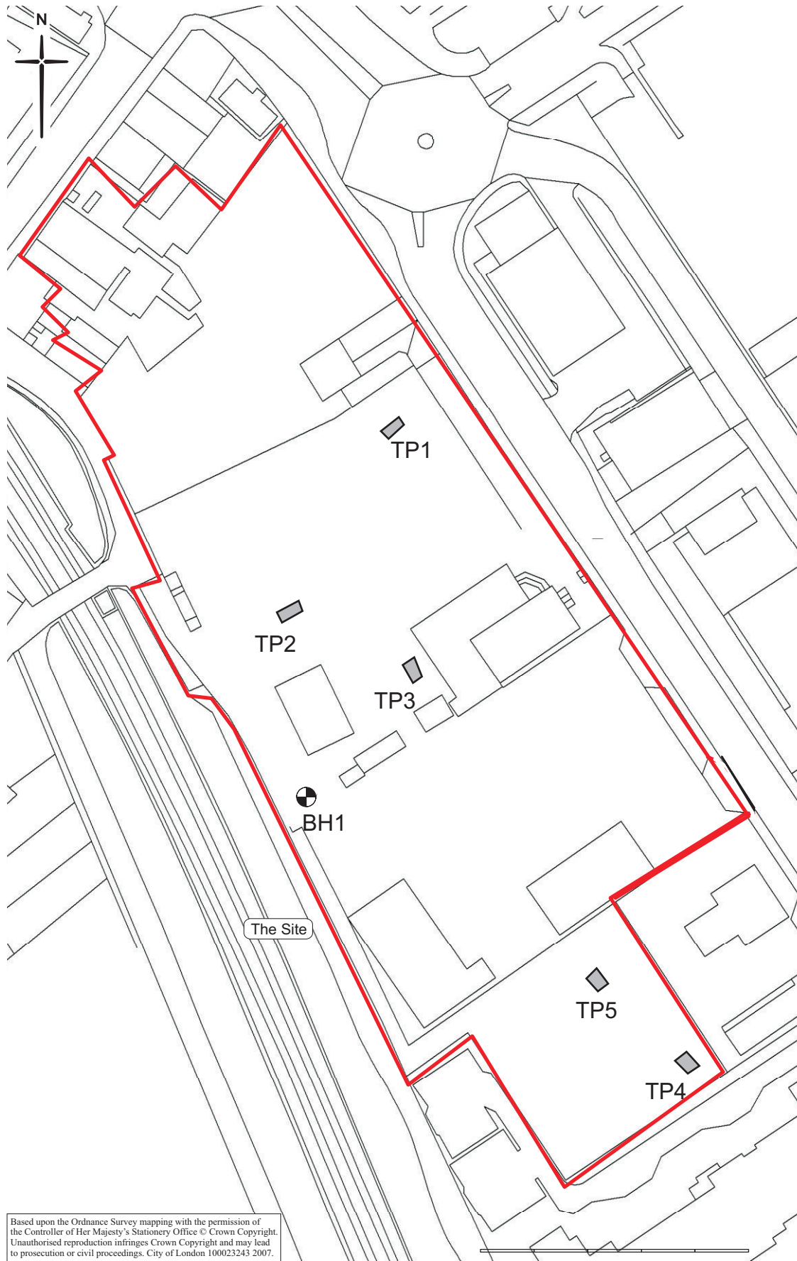
Fig 2 Location of trial pits and borehole
