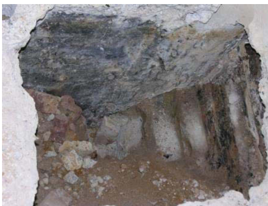
Fig 10 Trial pit 8 looking northwest Loose modern fill to the base of the trial pit 8.2m OD
