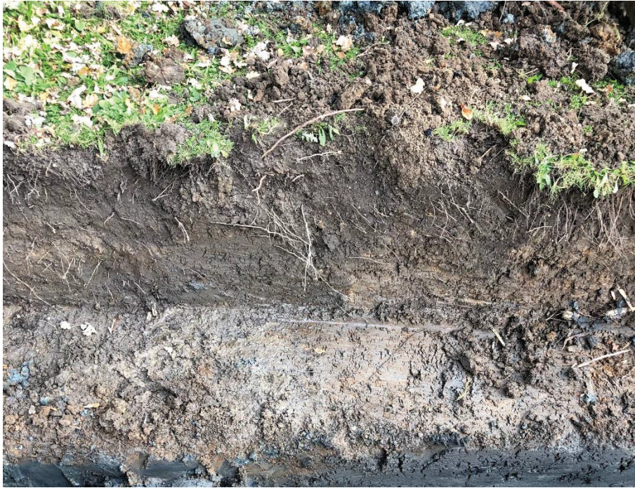
Photo 4: Approximately 1m thick brown made ground deposits over the lower blue grey clays; Trench 1 Valence House
