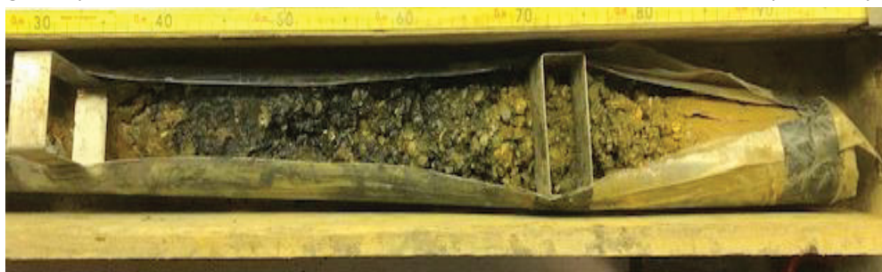
Photo 2: (L-R) Typical sequence of Hackney Gravels over London Clay deposits (BH_V2; Valence House)
