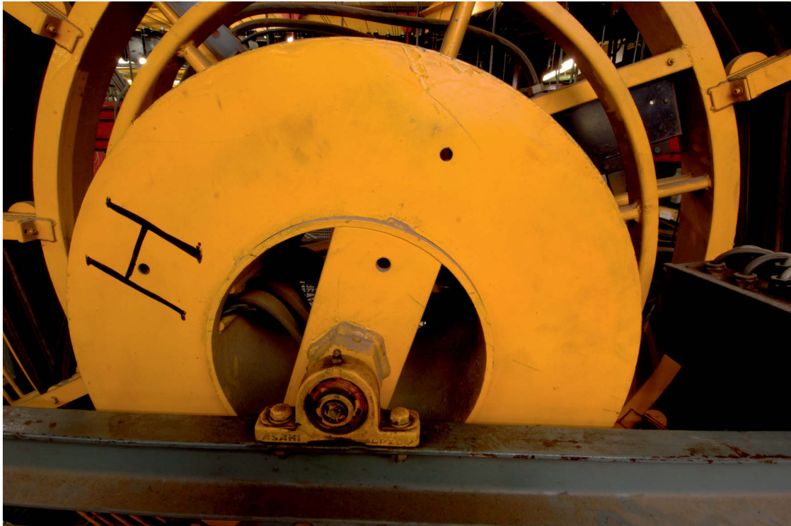
Fig 19 Detail of axle at front of windlass 5 (looking N, ie toward stage right), with hub of electricity supply reel (showing cable passing into centre of drum, from where it ran to lighting-cable reel)
