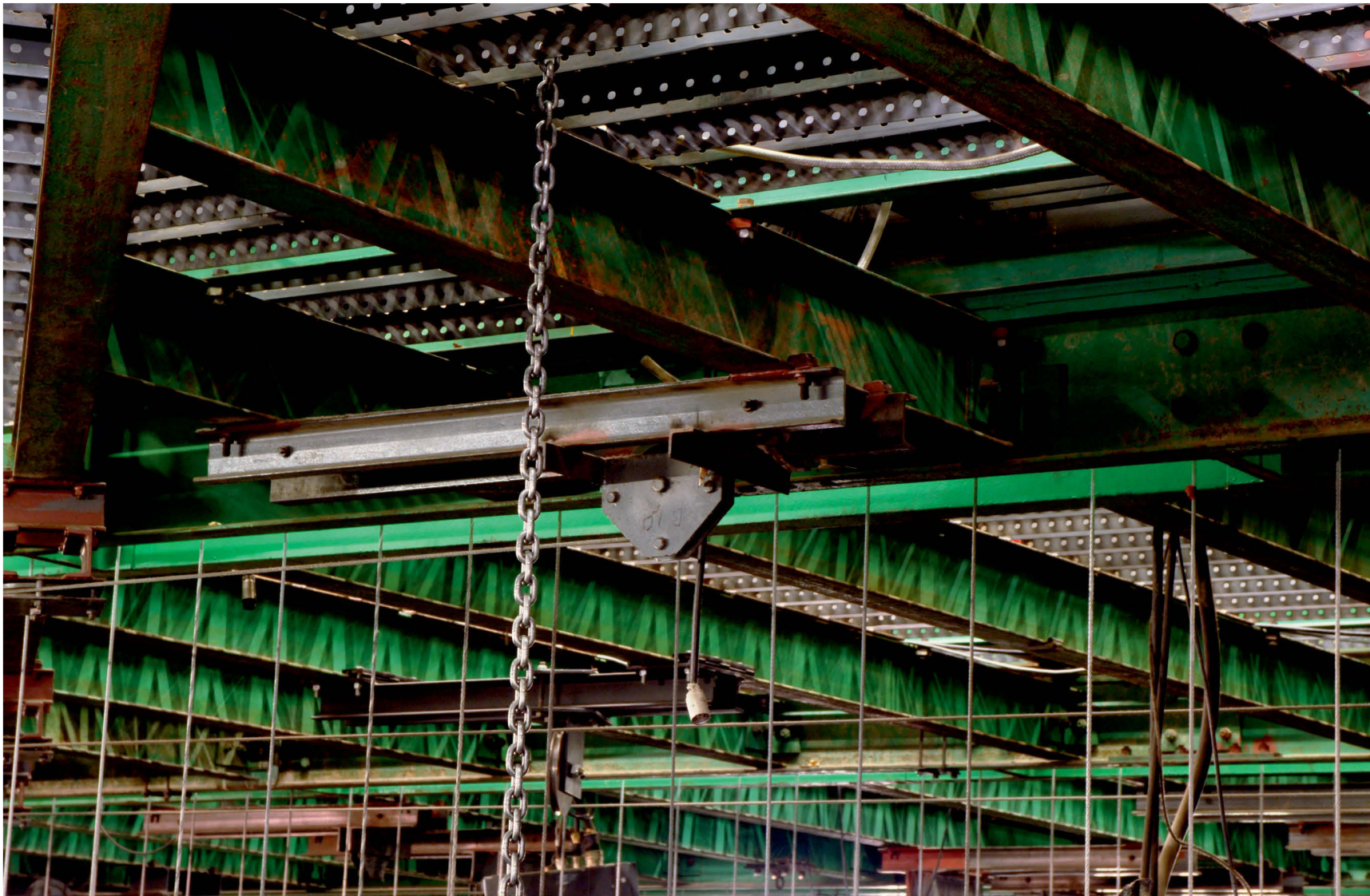
Fig 13 Looking up and to SE (ie upstage and toward the centre from stage right), showing the vertical diversion block below windlass 1 (suspended from the grid directly below the counterweight header block) – this block diverts the counterweight hauling line to run horizontally upstage, towards the back of the fly loft. A horizontal diversion block just visible at the extreme left diverts the line toward the array of loft blocks as shown in Fig 2
