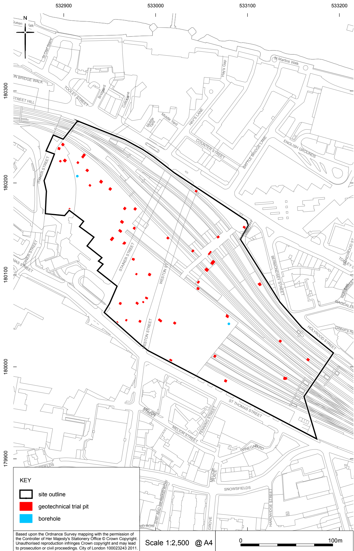
Fig 15 Key plan locating trial pits and boreholes
