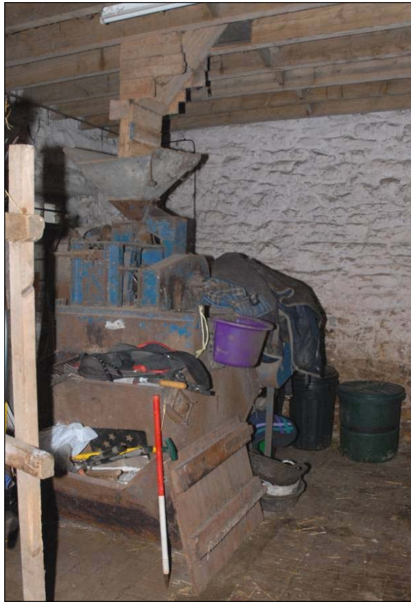
Unit 7, grain grinder with hopper from floor above, Fig 25
