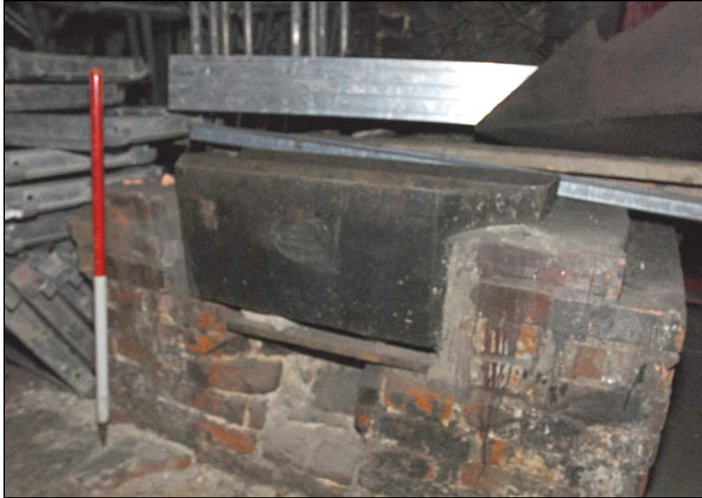
The hearth with the Alldays & Onions quenching tank
