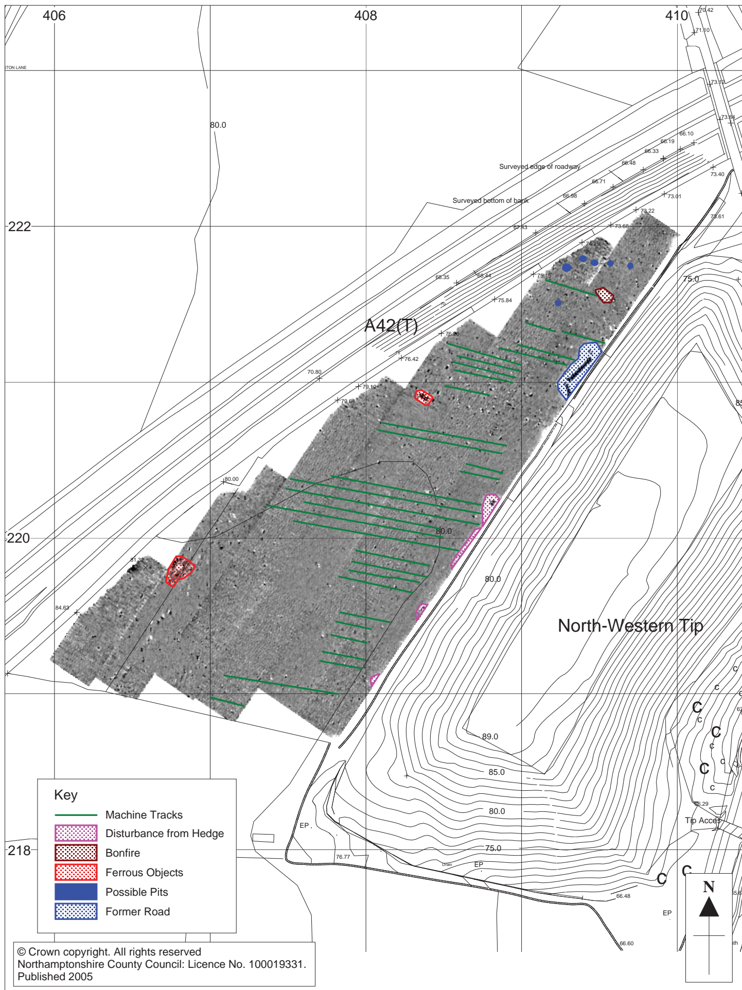
Figure 3 Detailed Gradiometer Survey Results with Interpretation
