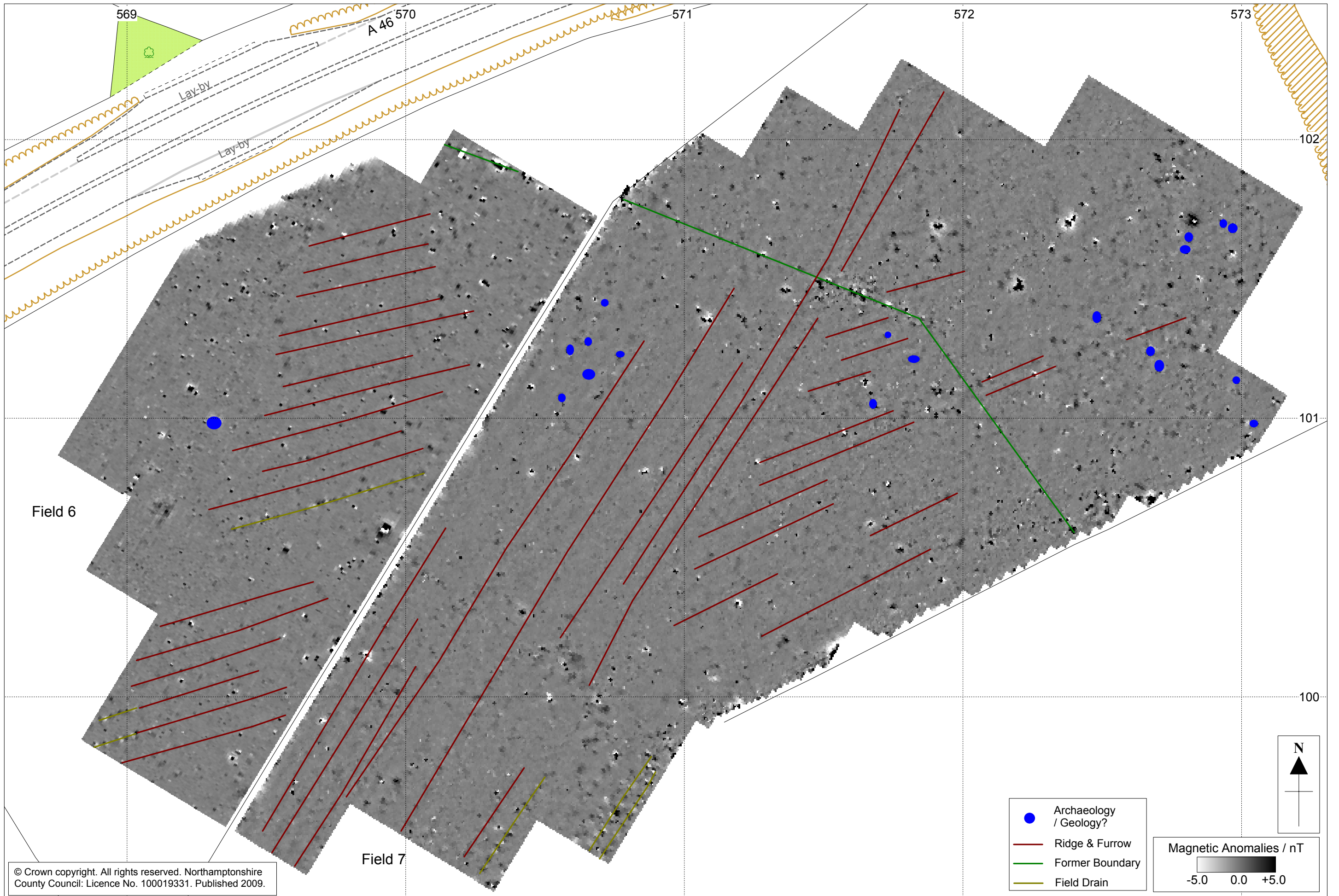
Gradiometer Survey Interpretation Fields 6 & 7 Fig 11
