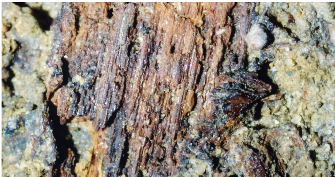
5 P9 b) Detail of organic remains in 5 P7 b) resembling wood/straw after exposure by airbrasive treatment
