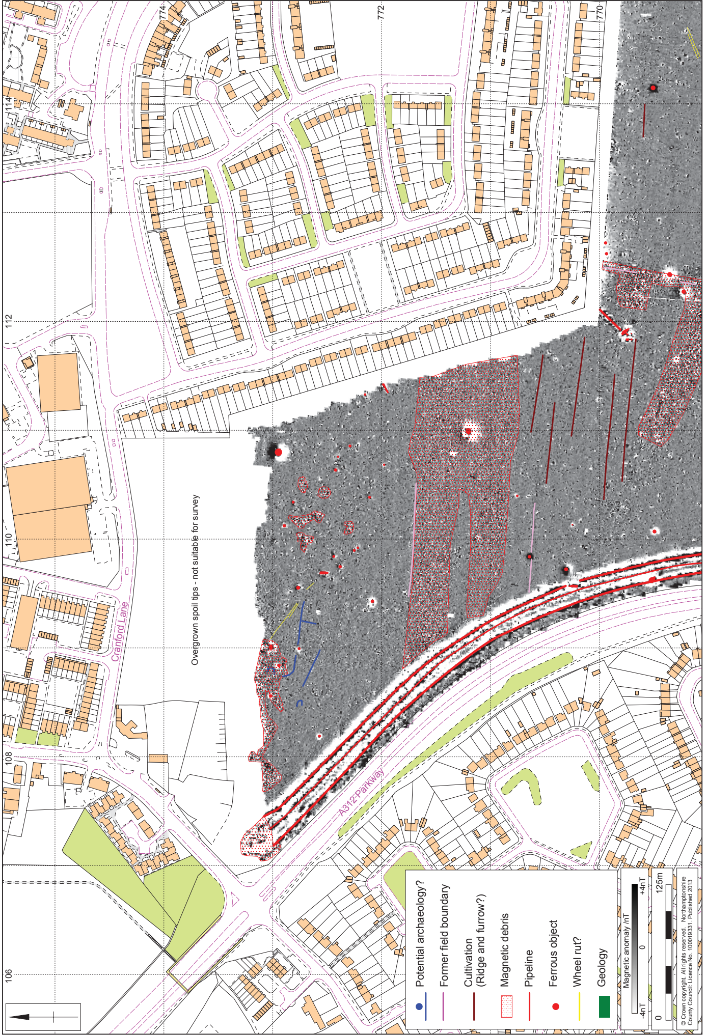
Magnetometer survey interpretation (North) Fig 3
