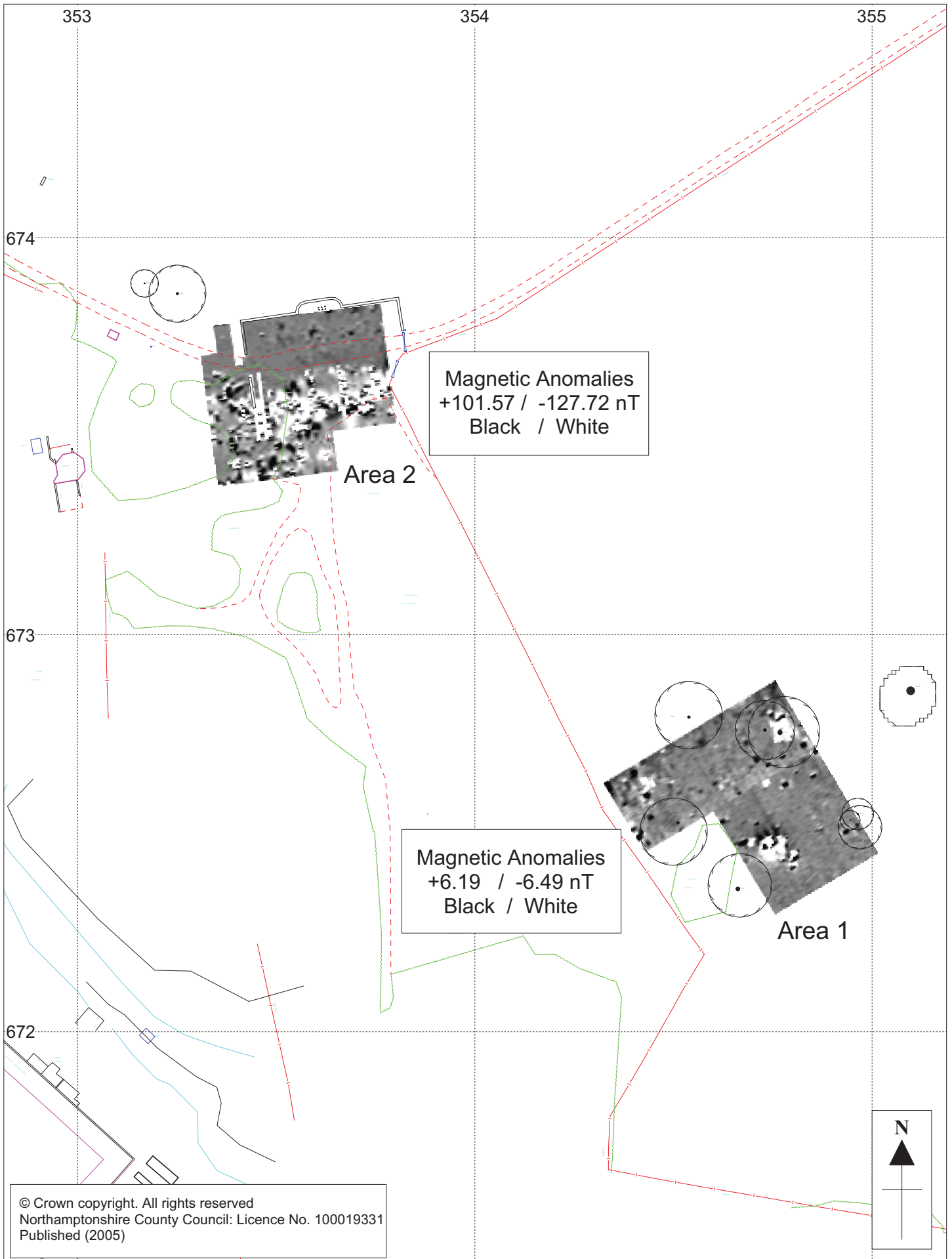
Fig 2 Detailed Gradiometer Survey Results
