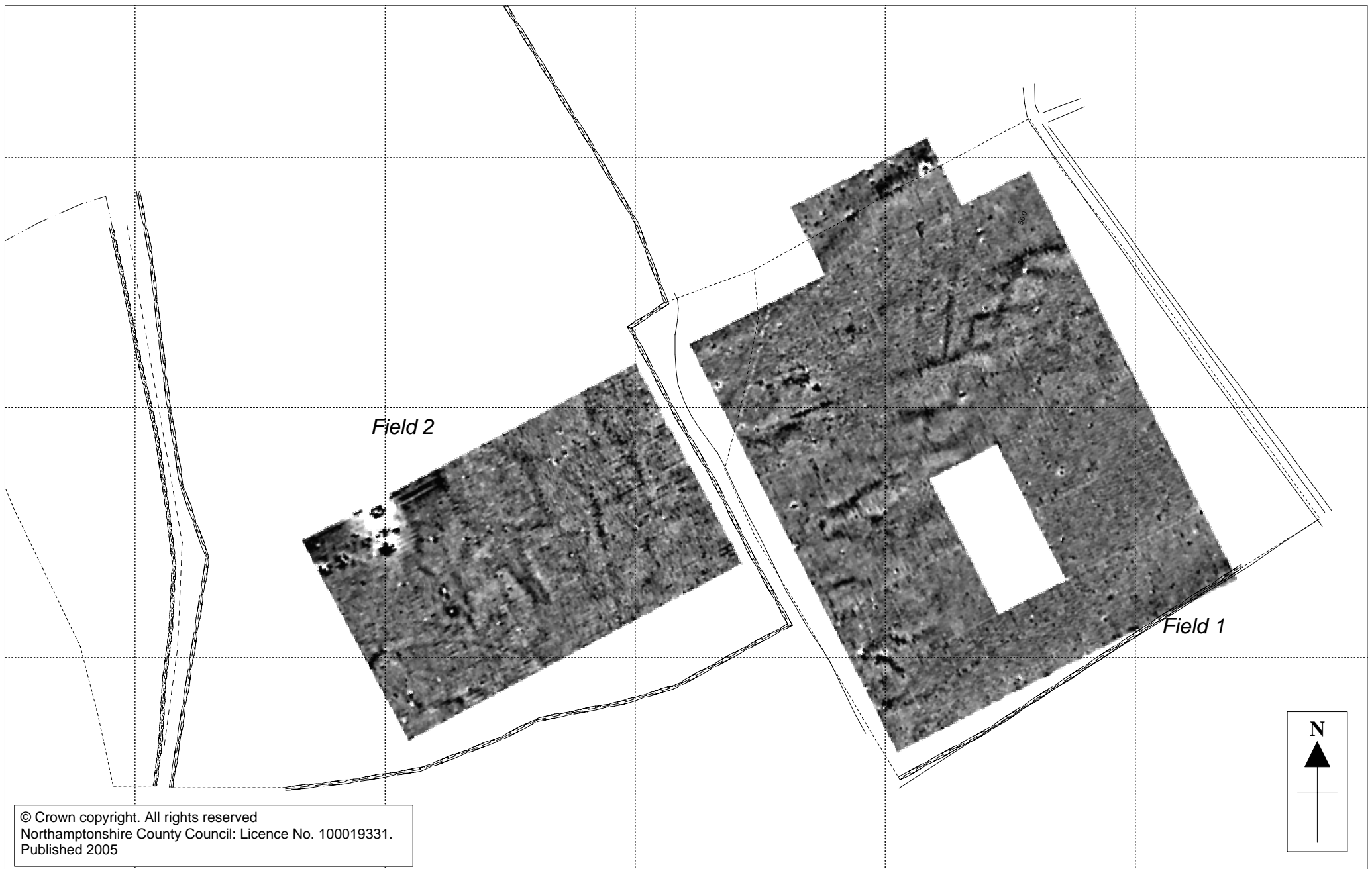
Figure 3: Gradiometer Survey Results Anomalies: -2.0nT / +1.0nT (white/black)
