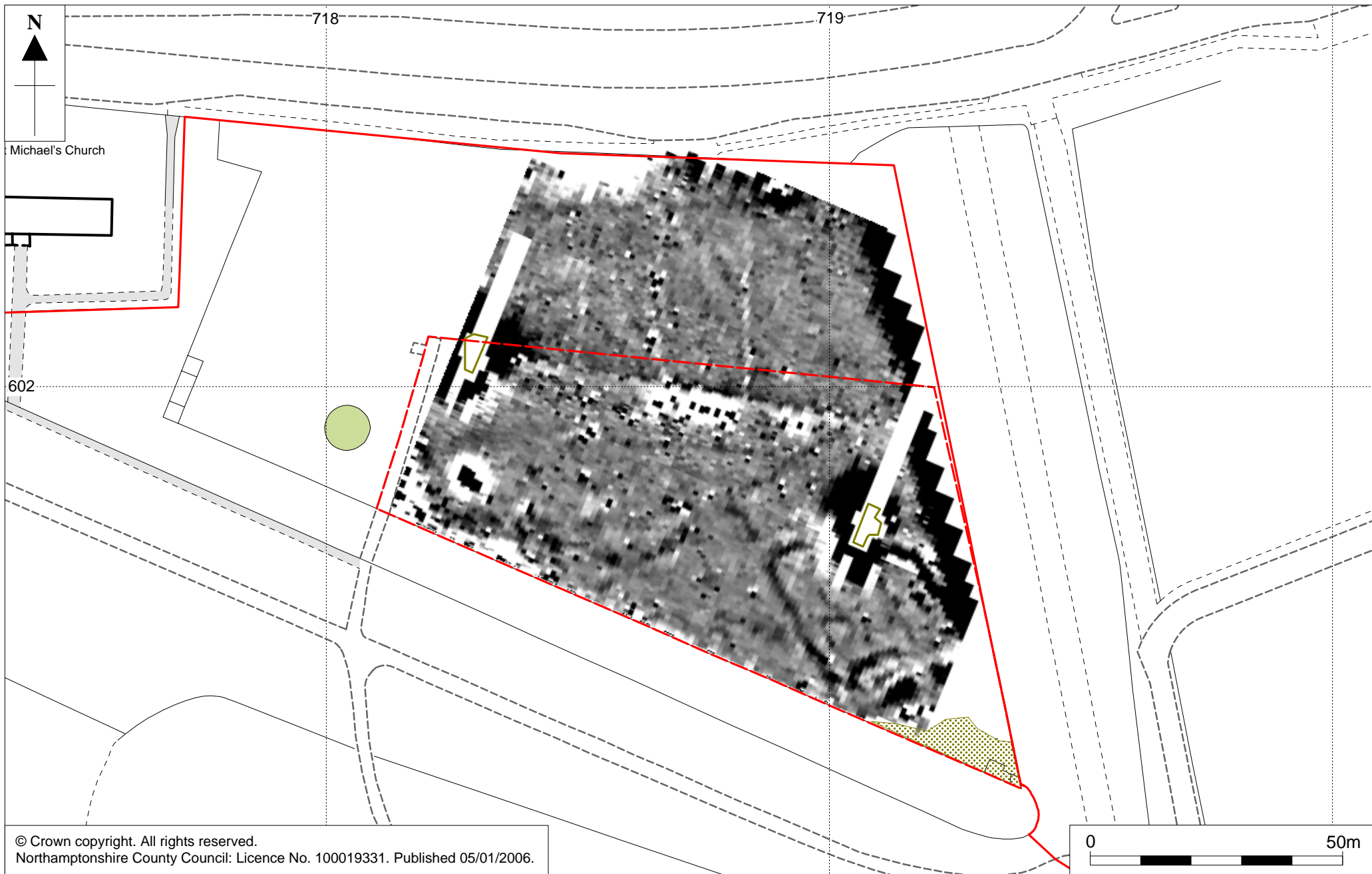
Fig 3 Gradiometer Survey Results -3nT / +3nT (white/black)
