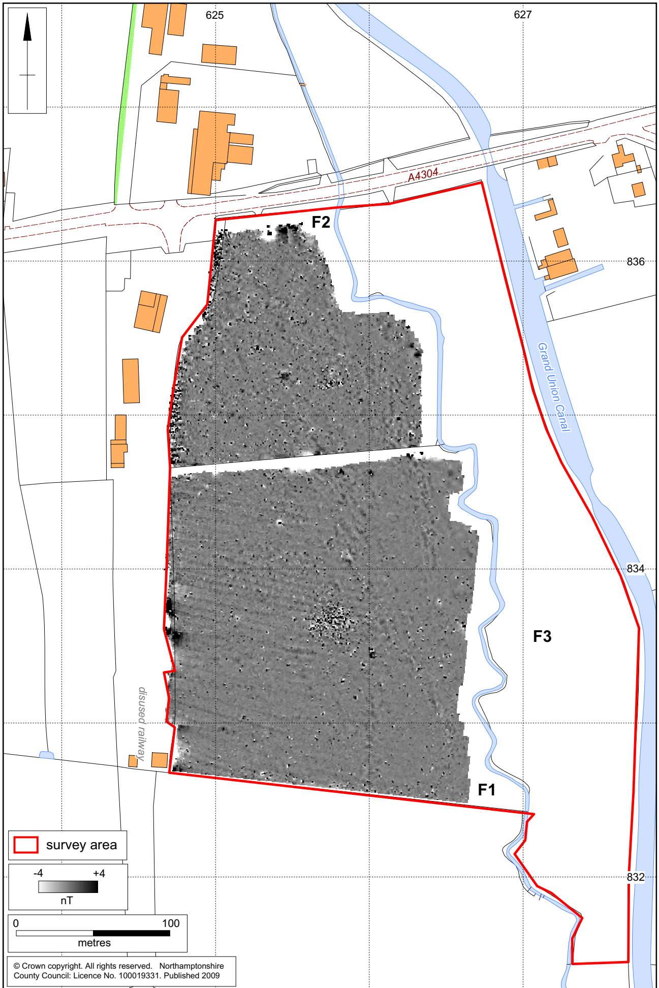
Magnetometer survey results, Fields 1 and 2 Fig 4
