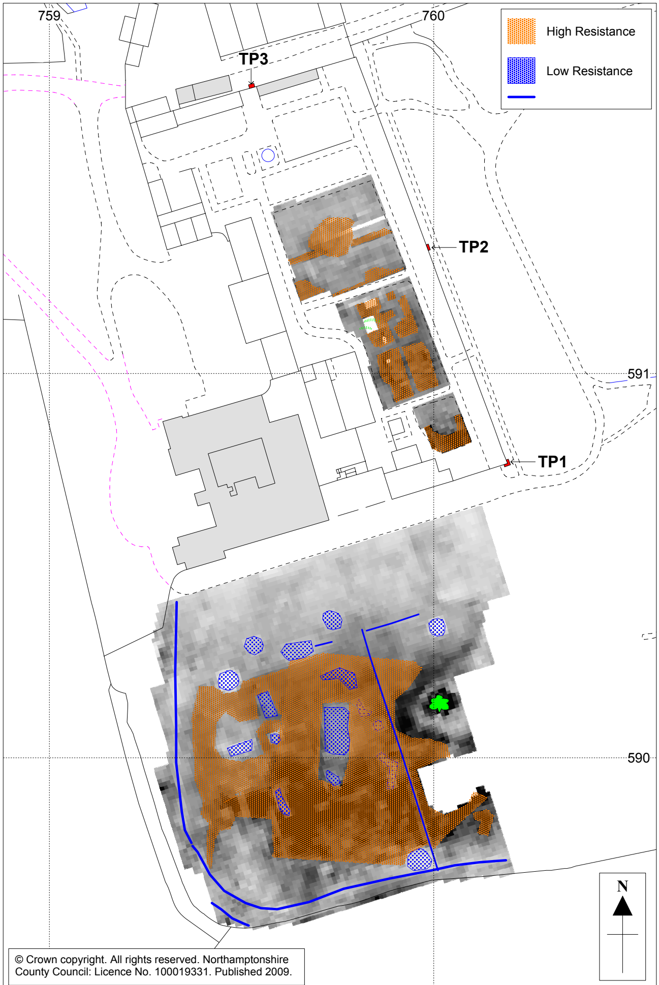
Earth Resistance Survey Interpretation and test pit location
