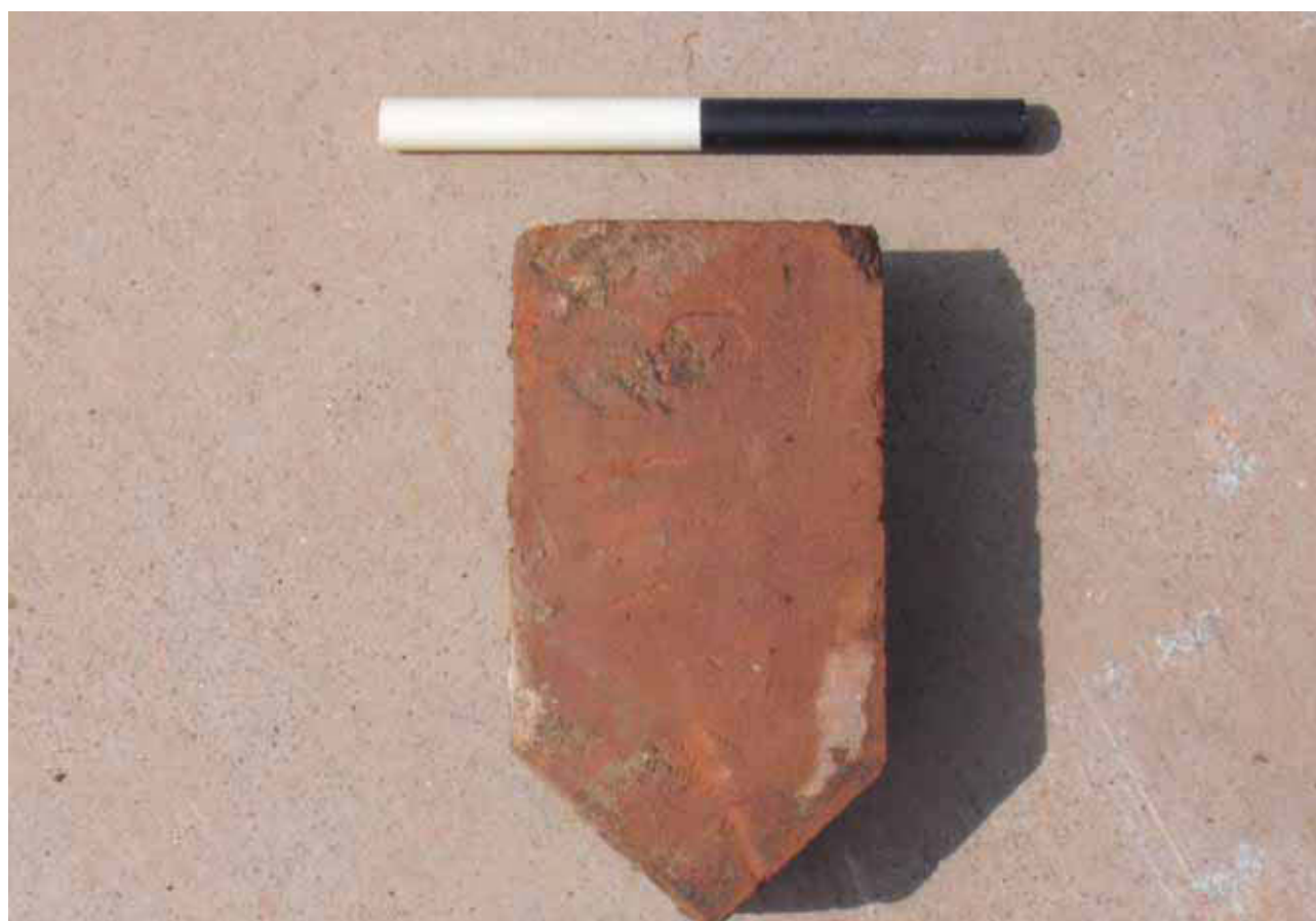
Fig 7 Shaped bricks used in the chevron-shaped sty entrance
