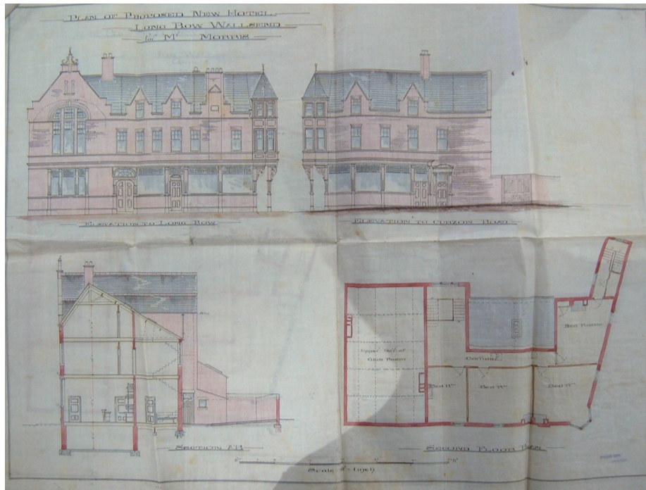
Plate 1b: Deposited Building Plans, 1892: Elevations, ground floor plan and section of Carville Hotel
