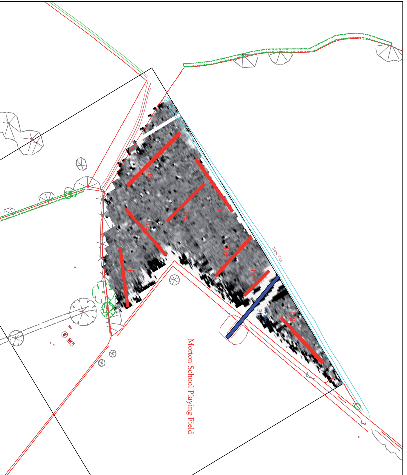
Figure 3 : Trench Location Plan (Overlaid on Geo-Physics Results)
