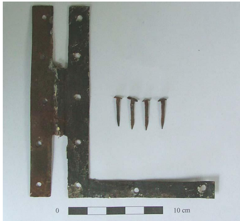
Plate 57 – One of the L-shaped hinges and associated nails removed from the bathroom door, second floor
