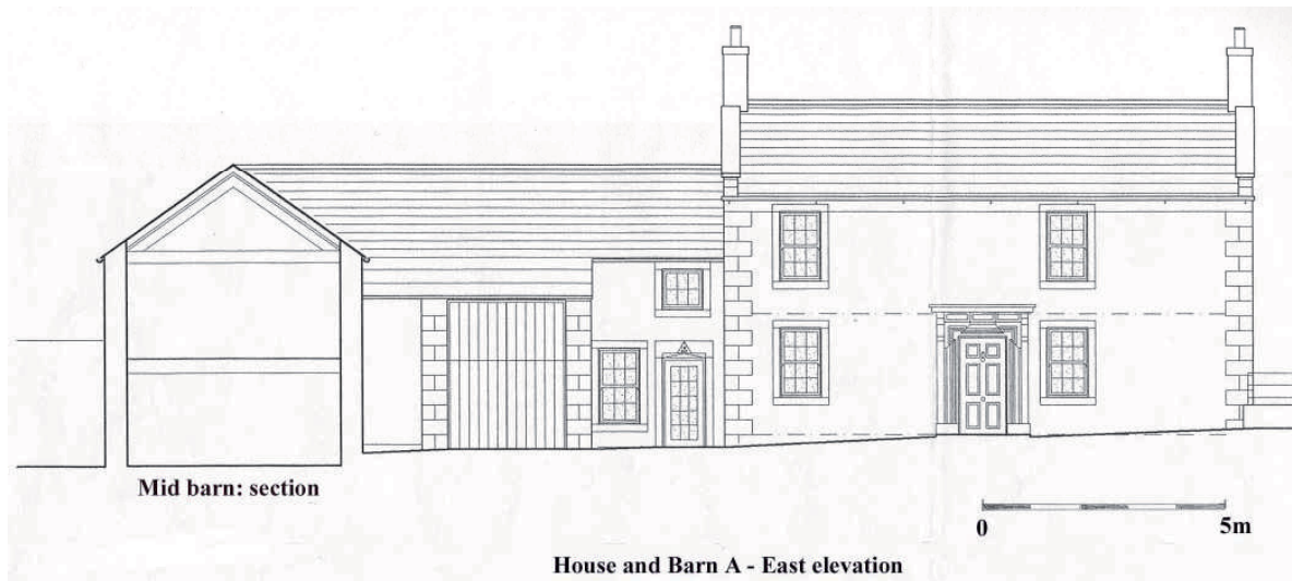
Figure 6 – East facing elevation of Barn A and House
