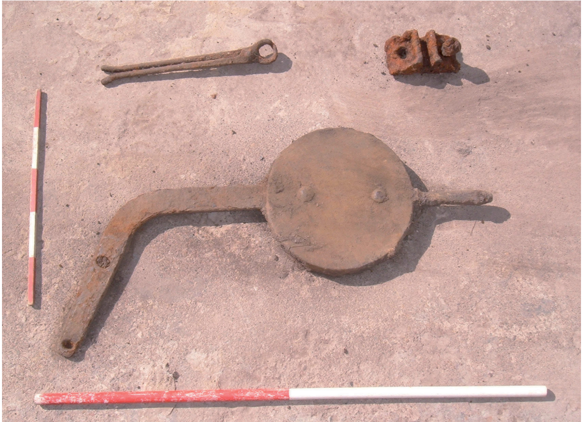
Plate 13: A points lever (SF 6), rail chair (SF 5) and large split pin (SF 7)
