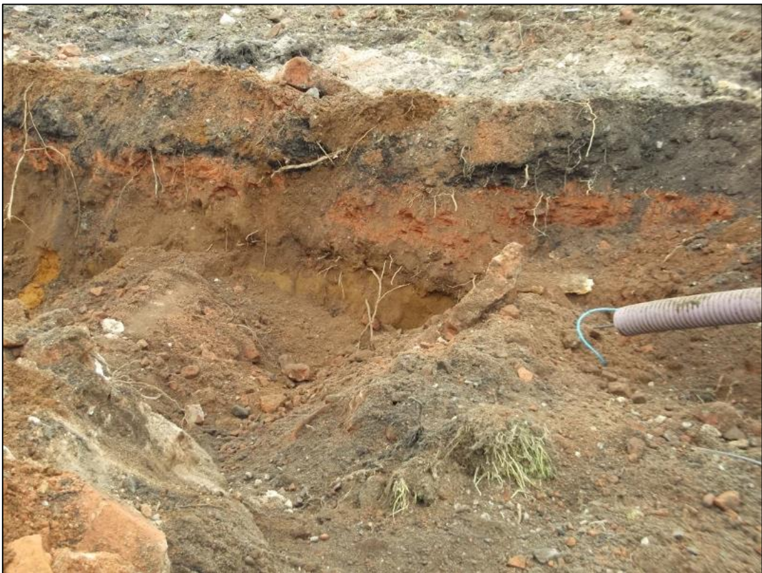
Figure 4b: Soil Profile, E side of Site (W-Facing) – detailed view of sediments
