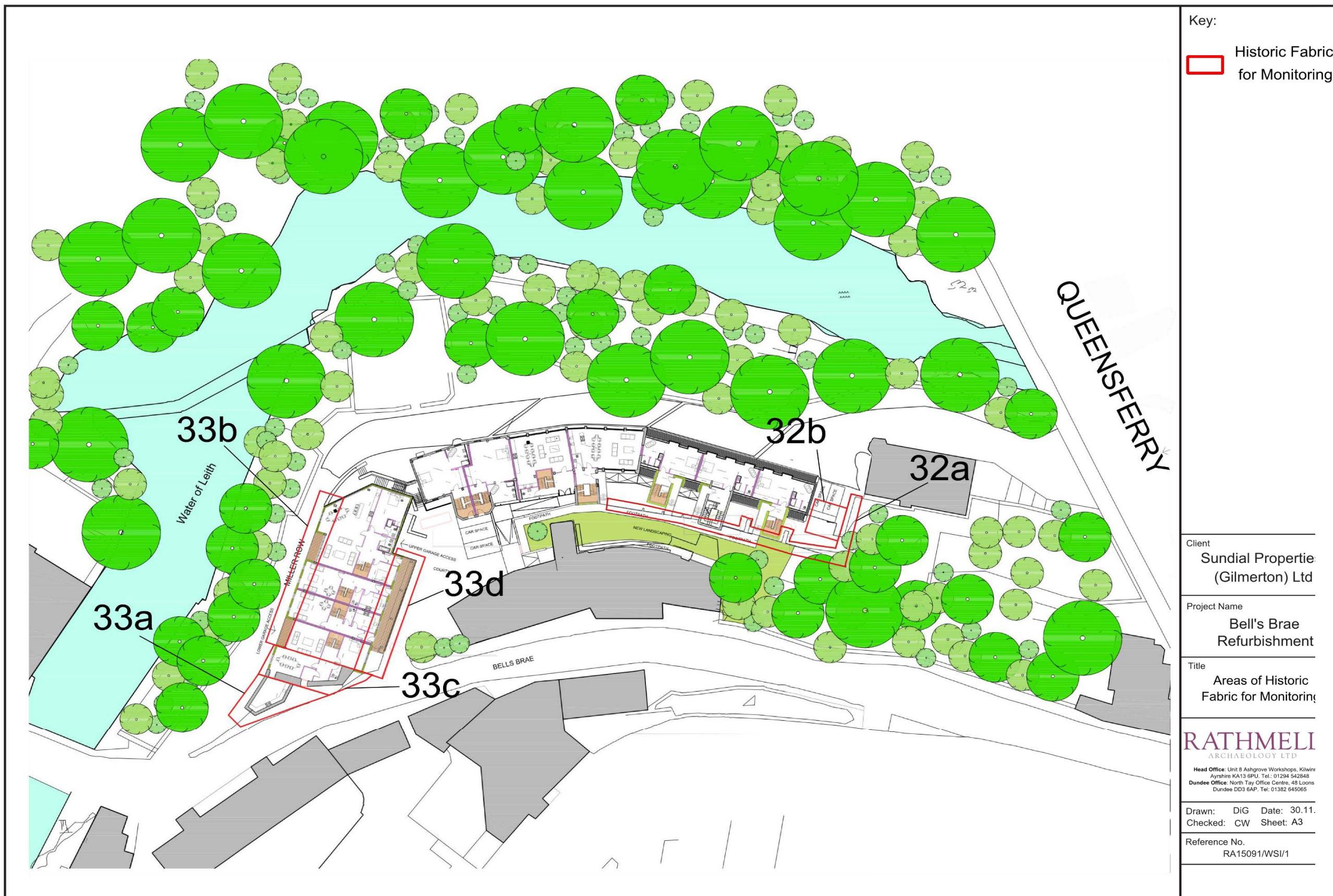
Figure 3: Plan of the development showing the areas of original structural fabric and monitored areas.
