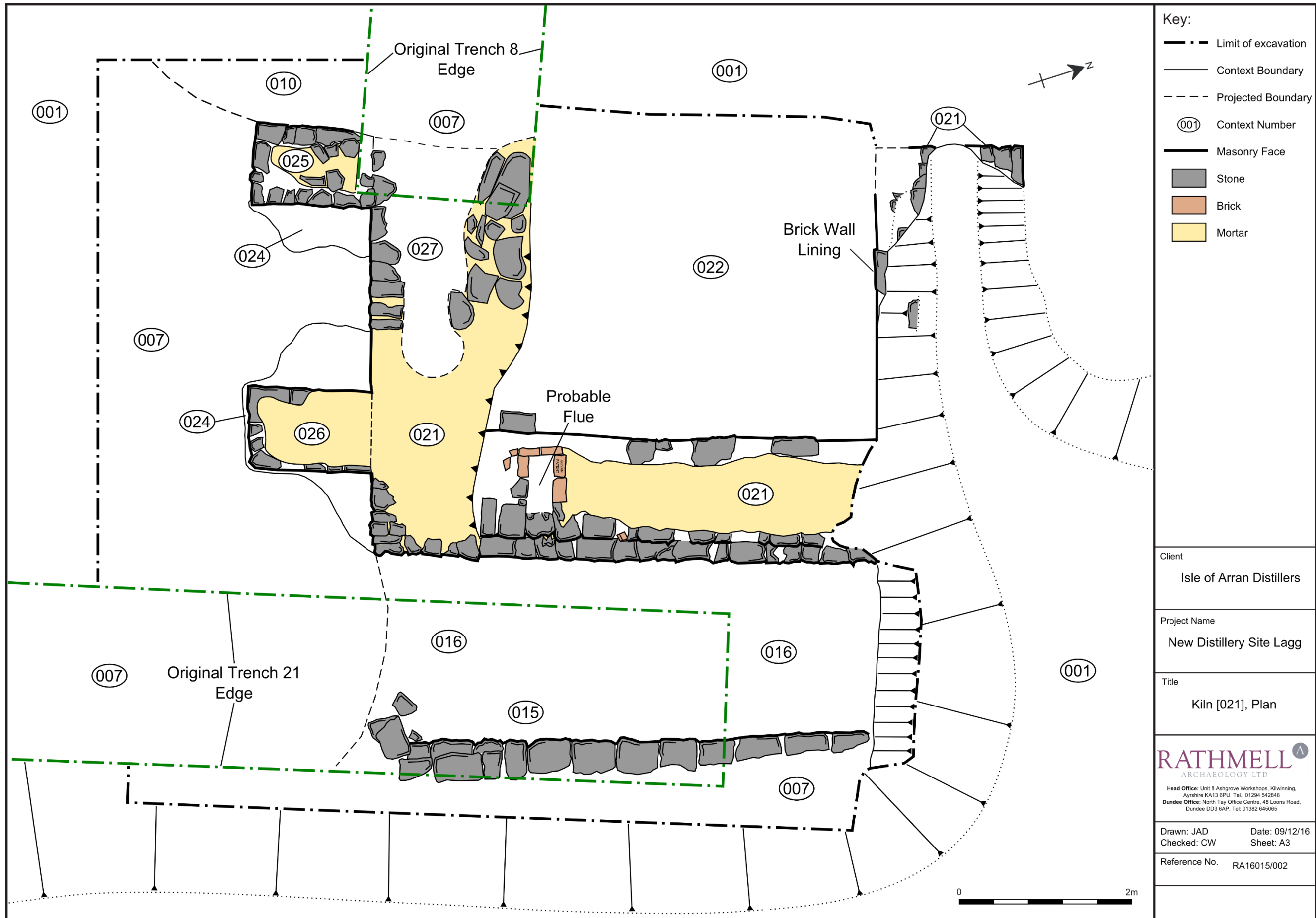
Figure 2: Plan of limekiln [021] and retaining wall [015].
